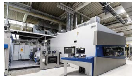
Surteco's new digital printing system can produce decor prints up to 225cm wide
